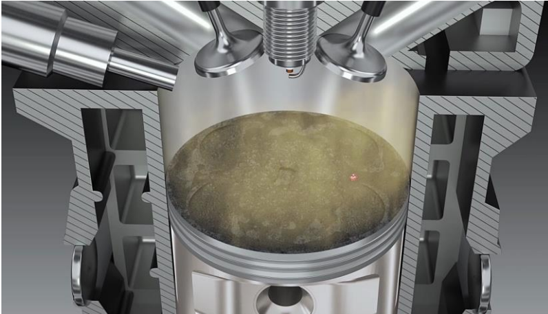
Illustration 1. A drop of oil detaches from the cylinder wall Source: TUNAP Group
