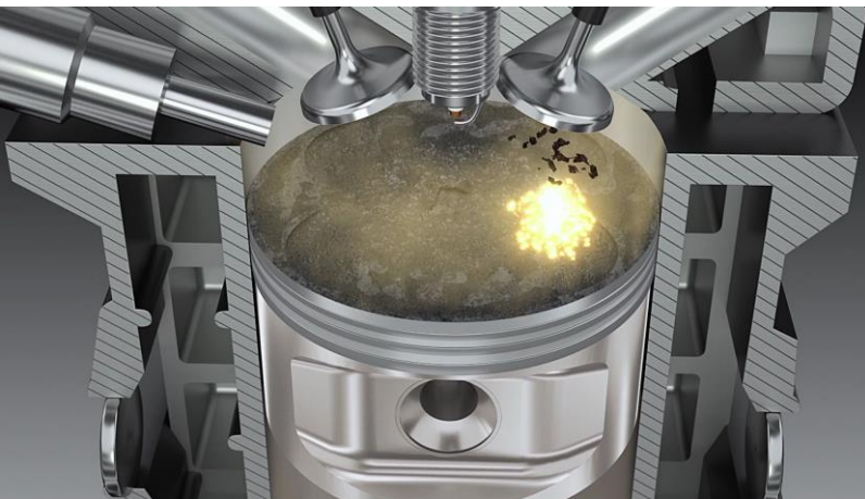
Illustration 2. Explosion of the drop of oil before ignition Source: TUNAP Group
